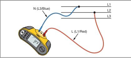
Figure 14. Measuring in a 3-Phase System
