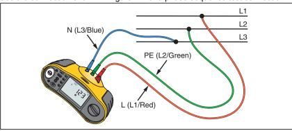
Figure 21. Phase Sequence Test Connection
