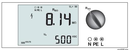
Figure 8. Insulation Resistance Display/Switch and Terminal Settings
