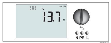
Figure 18. Earth Resistance Display/Switch and Terminal Settings
