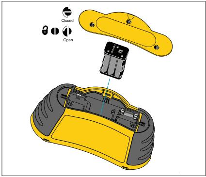
Figure 23. Replacing the Batteries
