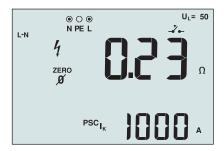
Figure 13. Line Impedance Display
