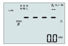
Figure 11. Display After Zeroing
