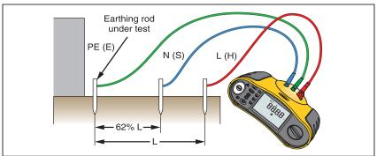
Figure 19. Earth Resistance Test Connection
