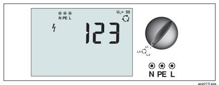
Figure 20. Phase Sequence Display/Switch and Terminal Settings
