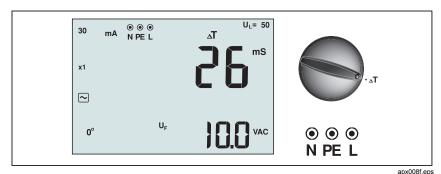
Figure 15. RCD Tripping Time Display/Switch and Terminal Settings
