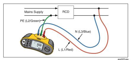
Figure 17. Connection for RCD Testing on IT Electrical Systems
