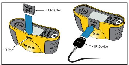
Figure 22. Attaching the IR Adapter
