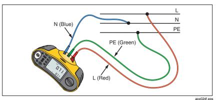
Figure 12. 3-Wire Connection for Earth Resistance Loop Test
