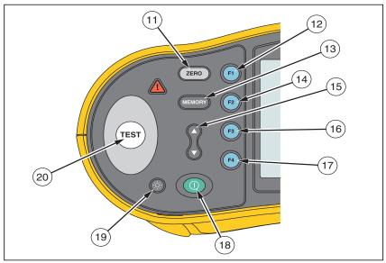
Figure 2. Pushbuttons
