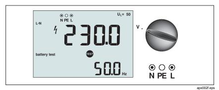
Figure 7. Volts Display/Switch and Terminal Settings
